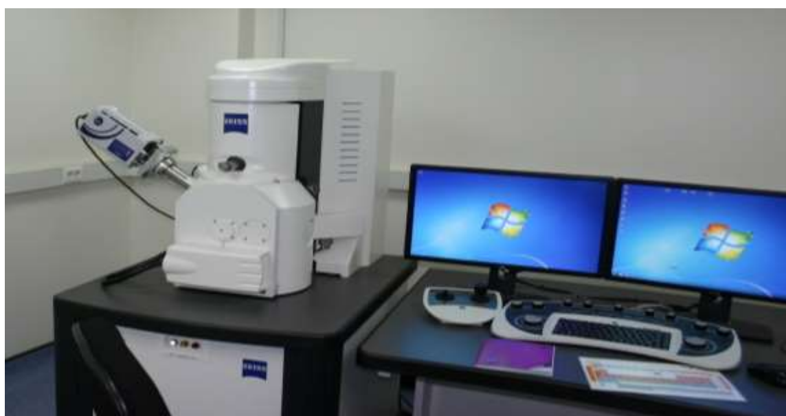
Fig. 46. Scanning electron microscope (EVOMA10(Oxford), Karl Zeiss)
